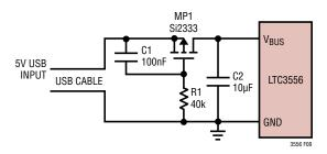
Figure 8. USB Soft Connect Circuit
