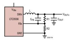
Figure 4. Buck Converter Application Circuit
