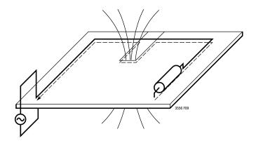
Figure 9. Higher Frequency Ground Currents Follow Their Incident Path. Slices in the Ground Plane Cause High Voltage and Increased Emissions
