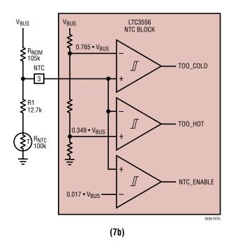
Figure 7. NTC Circuits
