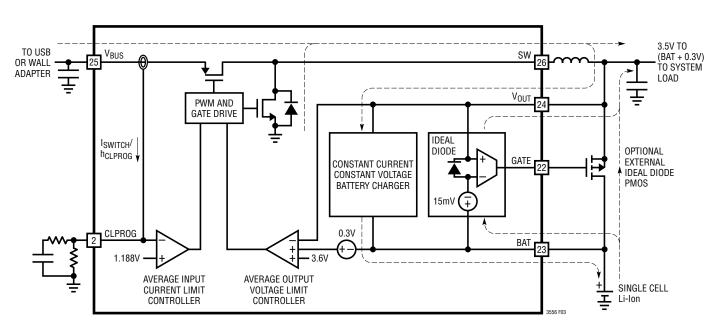
Figure 3. PowerPath Block Diagram
