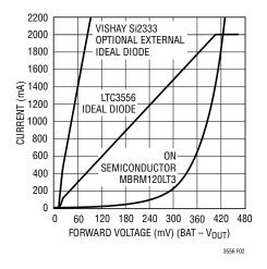
Figure 2. Ideal Diode Operation
