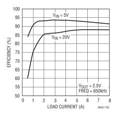
Figure 2. Efficiency vs Load Current of Figure 1
