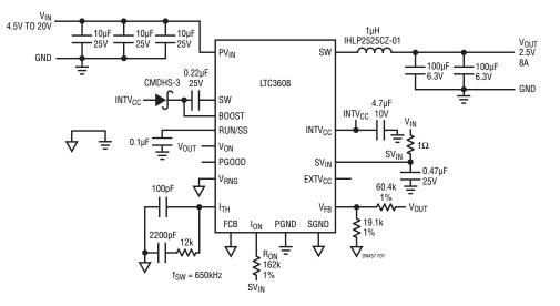
Figure 1. 4.5V to 20V Input to 2.5V/8A High Density Step-Down Converter
