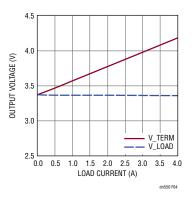
Figure 4. Cable Drop Operation Load Curves
