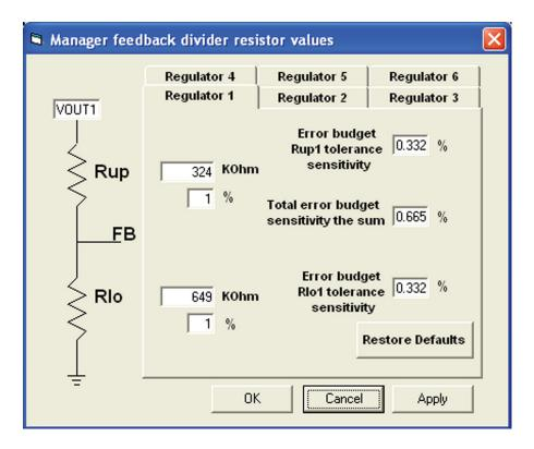
Figure 6. Change Resistor Divider Networks Window
