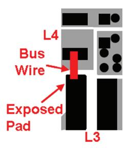
Figure 10. Buck3 and Buck4 Combined Setup
