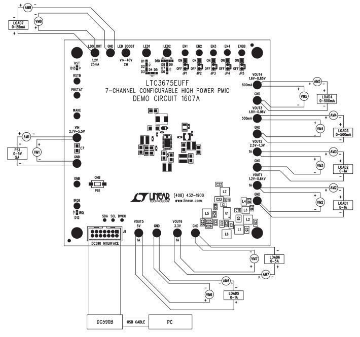
Figure 3. Proper Measurement Equipment Setup
