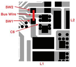
Figure 8. Buck1 and Buck2 Combined Setup
