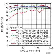
Boost Regulator, Efficiency vs Load
