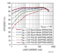
Buck-Boost Regulator, Efficiency vs Load
