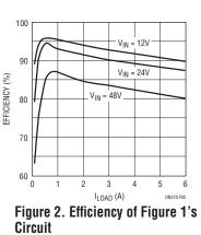
3.3V at 6A. The circuit can handle input transients up to 60V without requiring protection devices or 80V if appropriate MOSFETs are used. The frequency is set to 250kHz to optimize efficiency and output ripple. Figure 2 shows a mid-range efficiency of over 90% at
