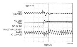
Figure 4. Line Transient Performance of Figure 1 Circuit Shows Almost Complete Rejection of 12V to 50V Supply Transient 24V input and 83.5% at 48V input. The loop is compensated for a 50kHz crossover frequency which provides 20 $\mu$ s response time to load transients (see Figure 3). The outstanding line transient performance is shown in Figure 4. The 12.1k R<sub>MAX</sub> resistor value is chosen to limit the inductor current to about 12A during a short-circuit condition.
