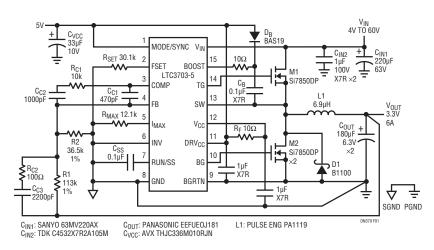
Figure 1. Buck: 48V to 3.3V/6A Synchronous Step-Down Converter
