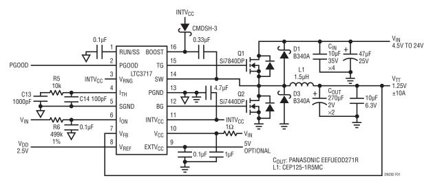
Figure 1. High Efficiency ±10A LTC3717  $V_{TT}$  Supply from 4.5V to 24V Input
