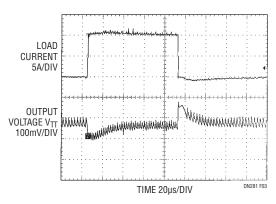
Figure 3. Load Transient Waveforms
