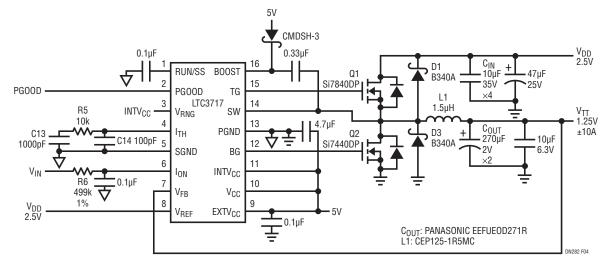
Figure 4. High Efficiency ±10A LTC3717  $V_{TT}$  Supply from  $V_{DD}$  Input
