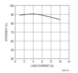
Figure 2. Measured Efficiency at 1.25V Output, 12V Input
