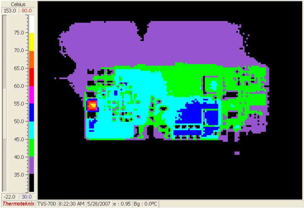
Figure 7. Thermal Map, Backside at 18Vin and 3.3Aout (Ta = 25 degrees C)
