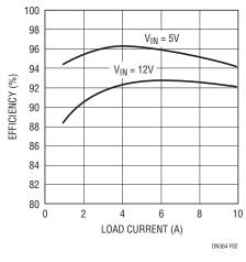
Figure 2. Efficiency Curves of the LTC3770 Converter in Figure 1
