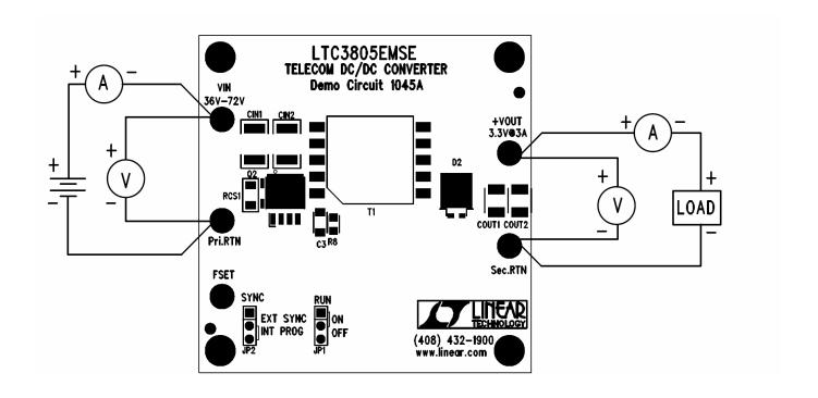
Figure 1. Proper Measurement Equipment Setup
