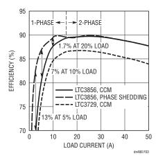
Figure 3. Efficiency Comparison:  $V_{IN} = 12V$ ,  $V_0 = 1.5V$ ,  $F_{SW} = 400$ kHz, L = 220nH,  $R_{SENSE} = 1m\Omega$ ,  $Q_T = RJK0305DPB$ ,  $Q_B = 2xRJK0330DPB$
