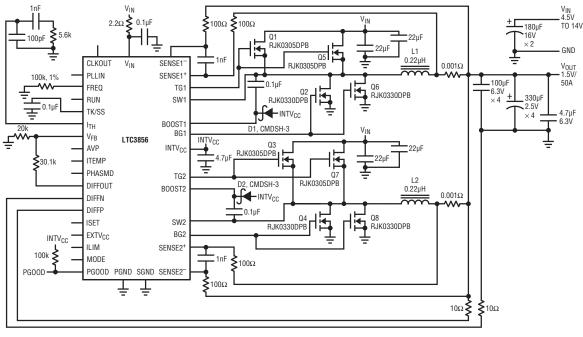
Figure 1. 1.5V/50A, 2-Phase Synchronous Buck Converter Featuring the LTC3856
