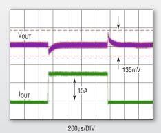
$12V_{IN},\,1.2V_{OUT},\,di/dt$  =  $100A/\mu s,\,f_{SW}\approx 400kHz$  OUTPUT CAP:  $2\times\,330\mu F$  POSCAP,  $2\times\,100\mu F$  CERAMIC
