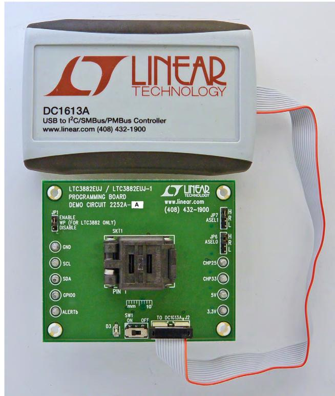
Figure 3. DC1613A Ribbon Cable Installation
