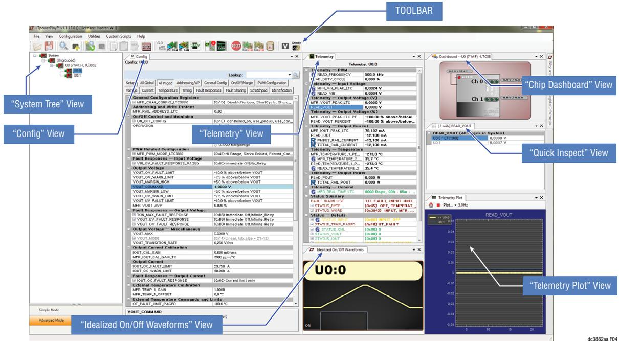
Figure 4. LTpowerPlay Interface of Programming the LTC3882
