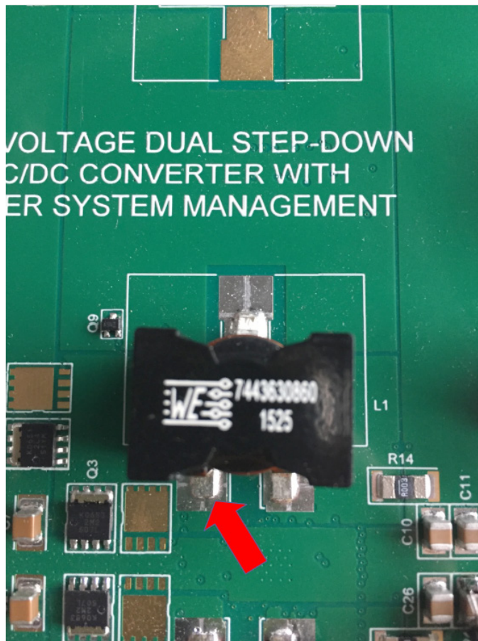
Figure 36. Probe Switching Node for Best Jitter Measurement
