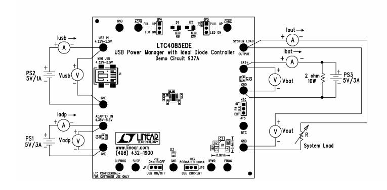
Figure 1. Proper Measurement Equipment Setup
