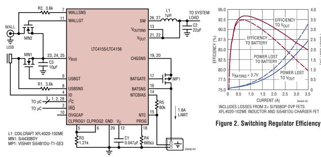
Figure 1. Typical Application Using a Simple Input Multiplexer with No Backdrive Protection
