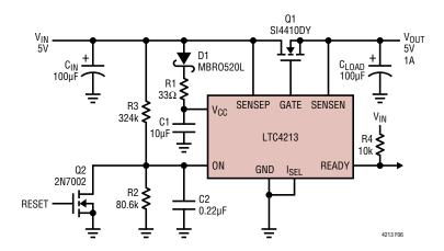
Figure 6. Single Supply Electronic Fuse
