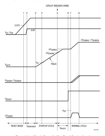
Figure 4. Load Supply Power-Up After Circuit Breaker Armed
