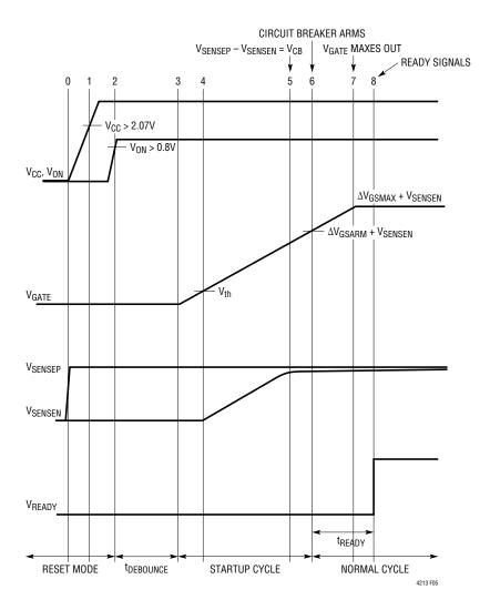
Figure 5. Load Supply Power-Up Before V<sub>CC</sub>
