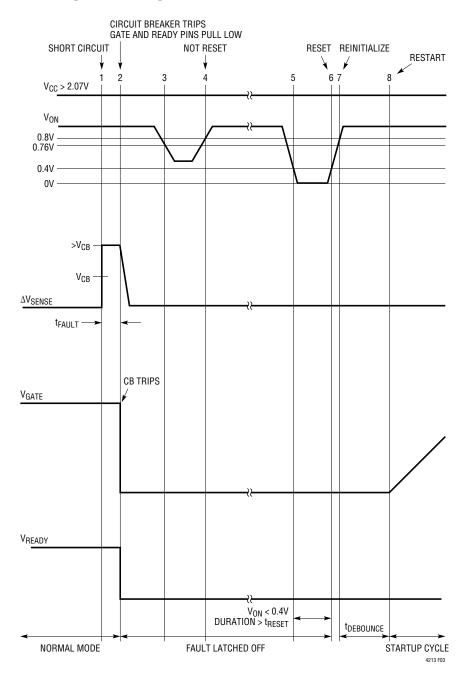
Figure 3. Resetting Fault Timing Diagram
