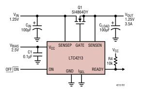
Figure 1. LTC4213 Electronic Circuit Breaker Application
