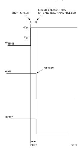
Figure 2. Short Circuit Fault Timing Diagram
