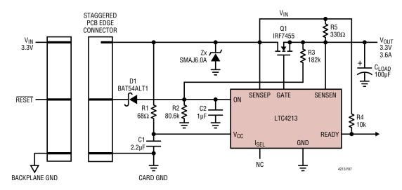
Figure 7. Single Supply Hot Board Insertion
