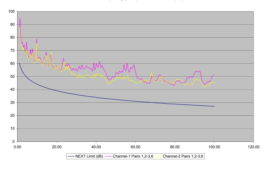
CAT 5 - TSB95 Spec @ Maximum Attenuation - Return Loss X-Axis Frequency (MHz), Y-Axis RL (dB)
