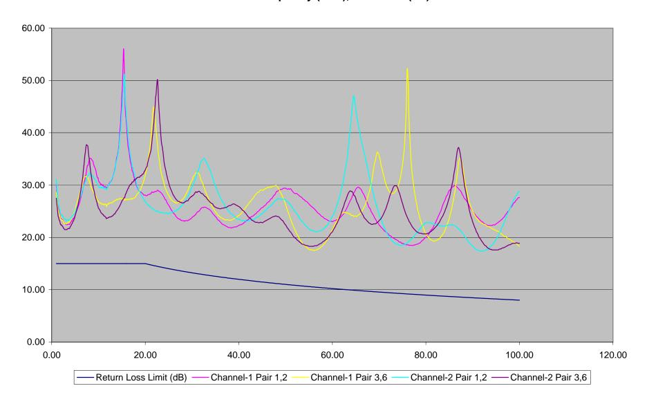
CAT 5 - TSB95 Spec @ Low Attenuation - Return Loss @ Remote X-Axis Frequency (MHz), Y-Axis RL-R (dB)
