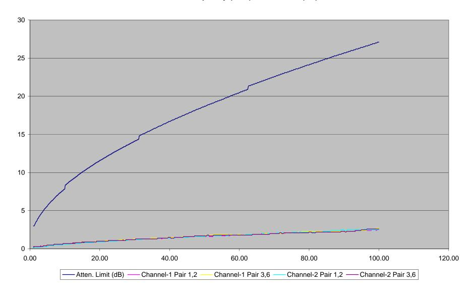
CAT 5 - TSB95 Spec @ Low Attenuation - Near End Cross Talk X-Axis Frequency (MHz), Y-Axis NEXT (dB)
