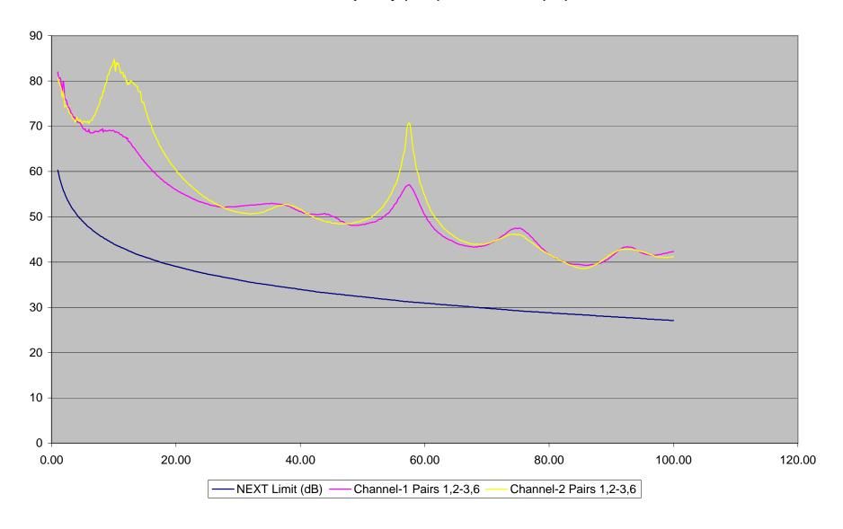
CAT 5 - TSB95 Spec @ Low Attenuation - Near End Cross Talk @ Remote X-Axis Frequency (MHz), Y-Axis NEXT-R (dB)
