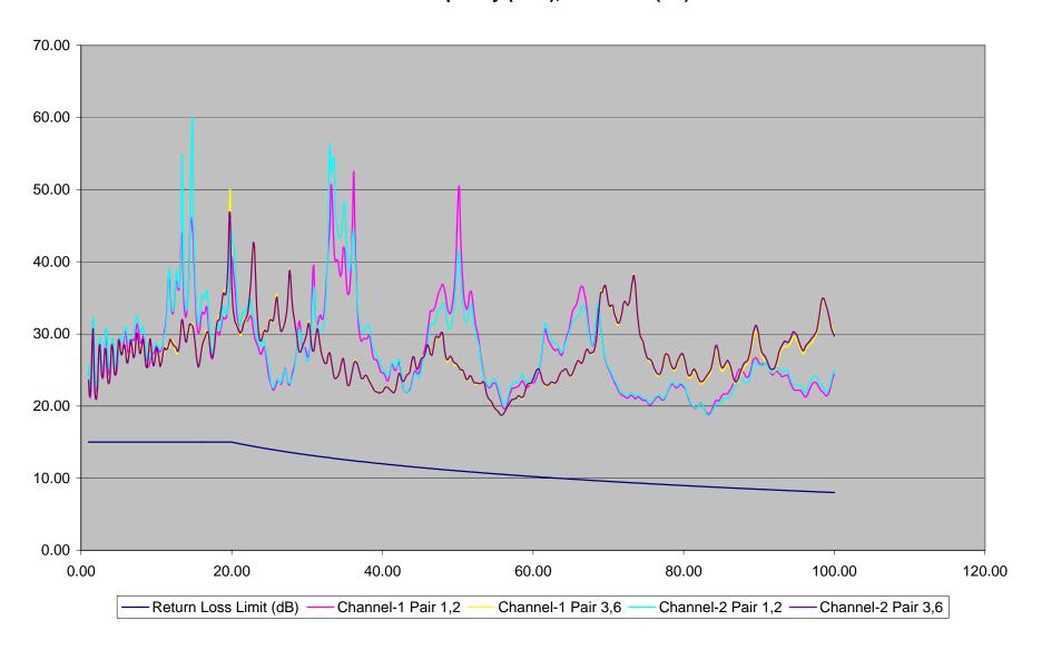
CAT 5 - TSB95 Spec @ Maximum Attenuation - Return Loss @ Remote X-Axis Frequency (MHz), Y-Axis RL-R (dB)
