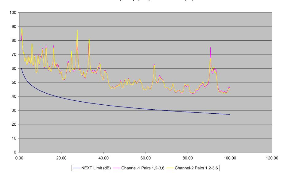
CAT 5 - TSB95 Spec @ Maximum Attenuation - Near End Cross Talk @ Remote X-Axis Frequency (MHz), Y-Axis NEXT-R (dB)
