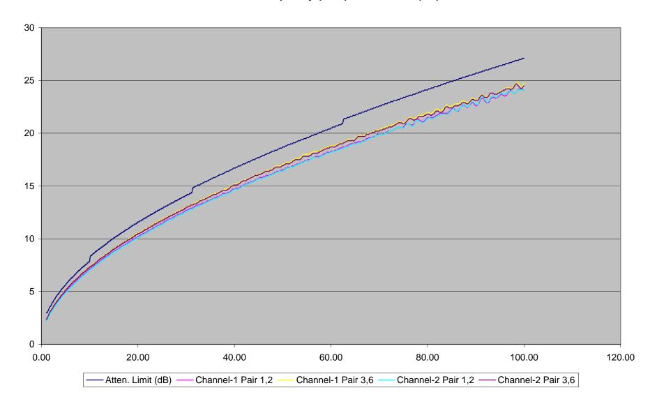
CAT 5 - TSB95 Spec @ Maximum Attenuation - Near End Cross Talk X-Axis Frequency (MHz), Y-Axis NEXT (dB)
