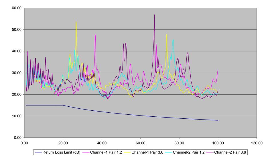
CAT 5 - TSB95 Spec @ Maximum Attenuation - Return Loss X-Axis Frequency (MHz), Y-Axis RL (dB)
