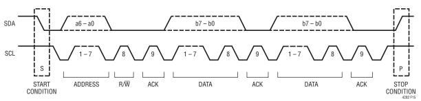
Figure 15. Data Transfer Over I<sup>2</sup>C or SMBus
