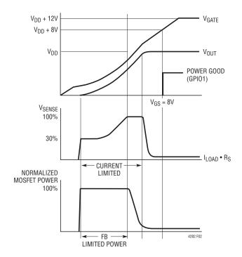
Figure 2. Power-Up Waveforms
