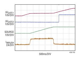
Figure 5. Normal Start-Up with Low Stress Staged Start
