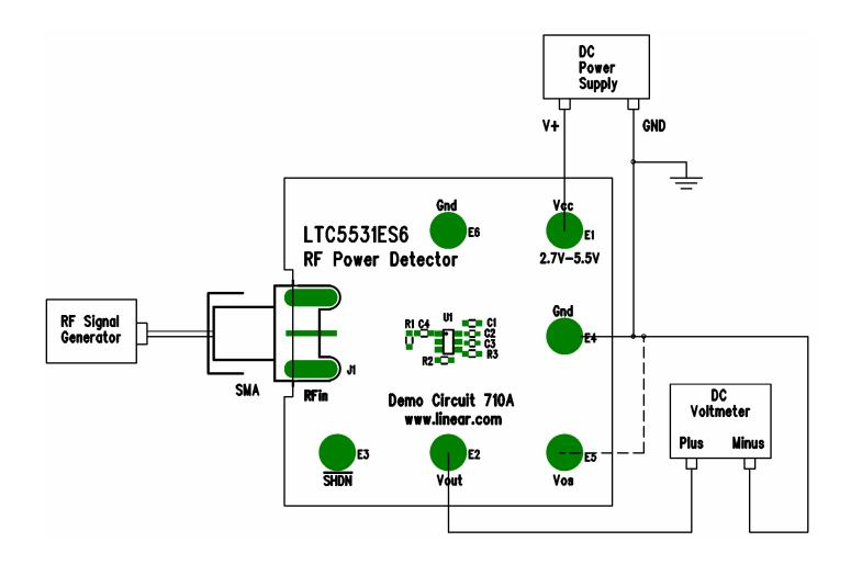
Figure 1. Proper Measurement Equipment Setup
