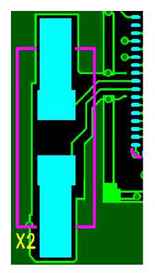
Figure 5. PCB Top Metal Layer Shielding of Crystal Signals
