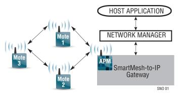
An ongoing discovery process ensures that the network continually discovers new paths as the RF conditions change. In addition, each mote in the network tracks performance statistics (e.g., quality of used paths and lists of potential paths) and periodically sends that information to the network manager in packets called health reports. The network manager uses health reports to continually optimize the network to maintain >99.999% data reliability even in the most challenging RF environments.
