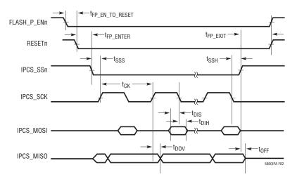
Figure 2. Flash Programming Interface Timing
