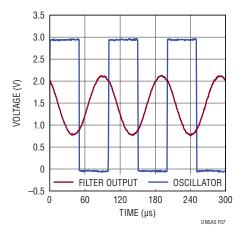
Figure 7. Voltage Waveforms Oscillator and Filter Output
