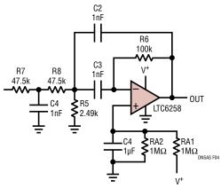
Figure 4. 10kHz Bandpass Filter
