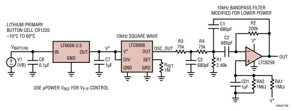
Figure 8. Oscillator and Filter with a Regulated Supply
