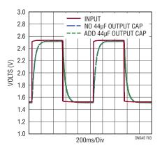
Figure 3. Reference Buffer Transient Response
