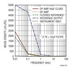
Figure 2. Buffer Noise Density
