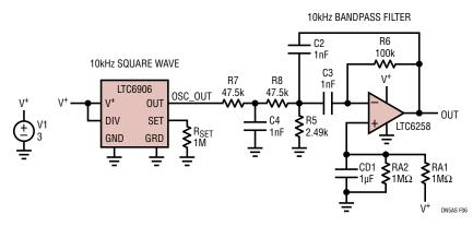
Figure 6. 10kHz Oscillator Circuit Using LTC6906 TimerBlox<sup>®</sup> Input
