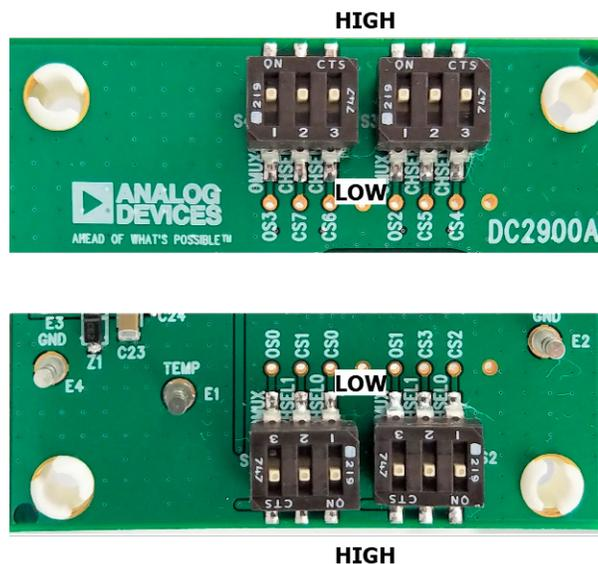
Figure 3. DC2900 Switch Positions for High and Low
