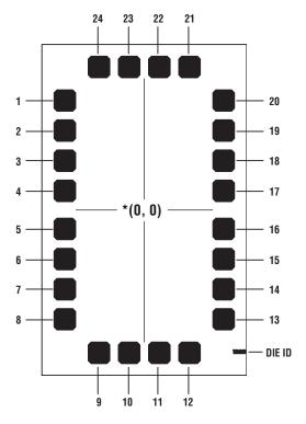
Die Size: 36mils (914.4µm)× 55mils (1397µm) Bond Pad Size: 4mils (102µm)× 4mils (102µm) Bond Pad Opening: 3.2mils (82µm)× 3.2mils (82µm) Bond Pad Metal Thickness: 0.29mils (7.4µm) Wafer Saw Street Width: 2.4mils (61µm) Wafer/Die Thickness: 8mils (200µm) Backside Metal: None Backside Potential: V<sup>-</sup>
