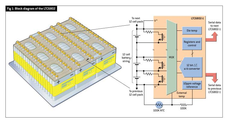
deliver significant power from an electrical system, such as during acceleration, hundreds of volts are required. Remember that delivering 1kW at 1V requires 1000A; delivering 1kW at 100V requires only 10A. Inherent resistance in system wiring and interconnects translates to IR loss, so designers use the highest voltage and lowest current that's practical.
