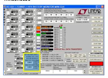
In the section labeled **SET VOLTAGE LIMITS** click on the boxes and enter voltage values for the over-voltage and under-voltage thresholds required for the cells being monitored. The voltage value entered will be rounded to the actual value used by the LTC6802-1 and displayed in the box. The voltage ranges for these thresholds is 0V to 5.12V and the program will not allow the under to be greater than the over voltage threshold.
