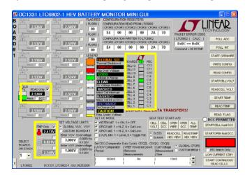
Each cell and each temperature channel has a check box to allow individual measurements. Checking these "Only" boxes sends the command (STARTCELL VOLT then READCELL VOLT, START TEMP then READ TEMP) to read only that channel and display its status. Cell 8 and Internal Temp are shown in the example screen above. Older or stale readings for all other cells and temperatures are faded out.
