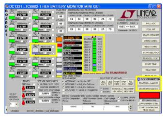
A check box is provided for each cell to be discharged. Checking this box (Cell 3 in the above example screen shot) and then writing the new configuration with a **WRITE CONFIG** button push will burden the cell.
