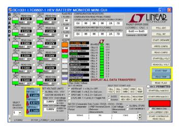
The LTC6802-1 has three ADC channels dedicated to measuring temperature. The temperature indications are for the internal die temperature of the LTC6902-1 and two externally connected thermistors. The display returns a voltage measurement.
