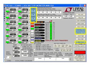
If the measured voltage of a cell is within the monitoring thresholds all indications for the cell appear green.
