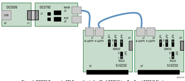
Figure 4. DC2792 Reverse isoSPI Connection to the "Top" DC2515 in a Two-Board DC2515 Stack
