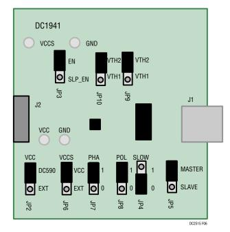
Figure 6. DC1941 isoSPI Master Mode Jumper Settings
