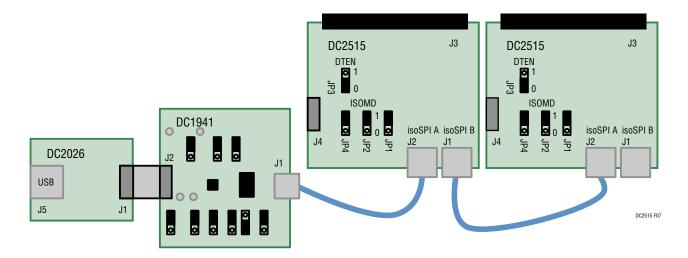
Figure 7. DC1941 Typical isoSPI Connection to the "Bottom" DC2515 in a Two-Board DC2515 Stack
