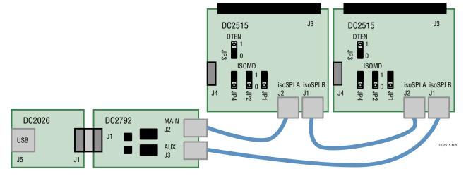
Figure 5. DC2792 Redundant isoSPI Connections to the "Bottom" and "Top" DC2515 in a Two-Board DC2515 Stack
