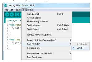
Select the correct Arduino compatible microcontroller board. Under the Tools menu, select Board → Arduino/ Genuino Uno with the "●" black dot symbol.
