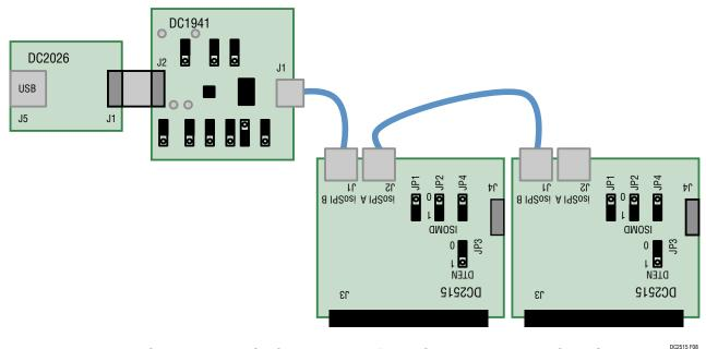
Figure 8. DC1941 Reverse isoSPI Connection to the "Top" DC2515 in a Two-Board DC2515 Stack
