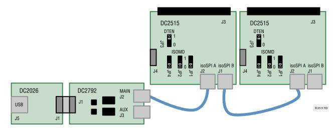
Figure 3. DC2792 Typical isoSPI Connection to the "Bottom" DC2515 in a Two-Board DC2515 Stack
