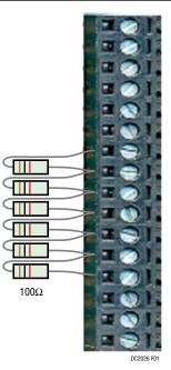
Figure 1. Resistor Divider String
