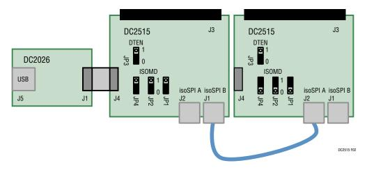
Figure 2. DC2026 SPI Connection to the "Bottom" DC2515 in a Two-Board DC2515 Stack
