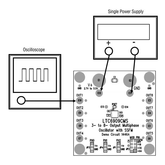
NOTE: The 6909 outputs (OUT1-OUT8) can drive 1k and 50pF loads. If a spectrum analyzer is used to measure the spread spectrum bandwidth then use a high impedance probe to monitor the outputs (typically the input impedance of a spectrum analyzer is 50 ohms).
