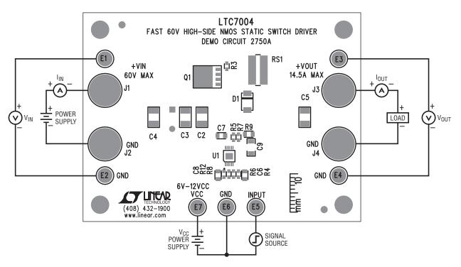
Figure 1. Proper Measurement Equipment Setup
