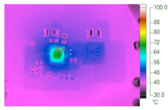
Conditions:  $48V_{IN}$ ,  $5V_{OUT}$  at  $2.3A_{OUT}$
