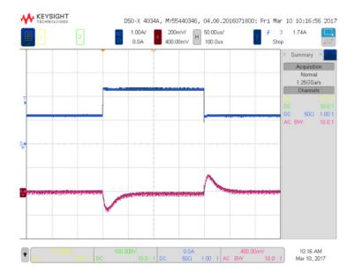
Figure 6. Transient Response Waveform at 48V<sub>IN</sub>, 5V<sub>OUT</sub> and 1.1A<sub>OUT</sub> to 2.3A<sub>OUT</sub> to 1.1A<sub>OUT</sub> (1A, 200mV, 50µs/DIV, 20MHz Bandwidth)
