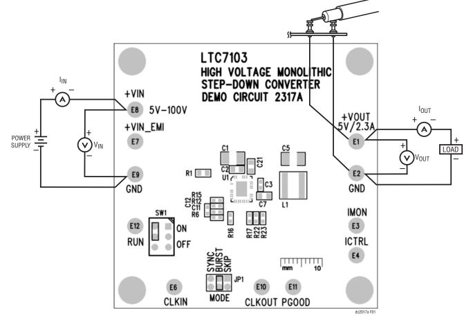
Figure 1. Proper Measurement Equipment Setup
