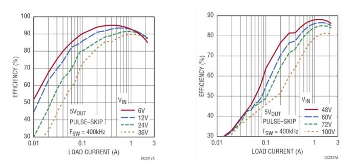
Figure 4. Efficiency at Various Input Voltages (Conditions: Pulse-Skipping Mode)
