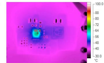
Conditions:  $24V_{IN}$ ,  $5V_{OUT}$  at  $2.3A_{OUT}$
