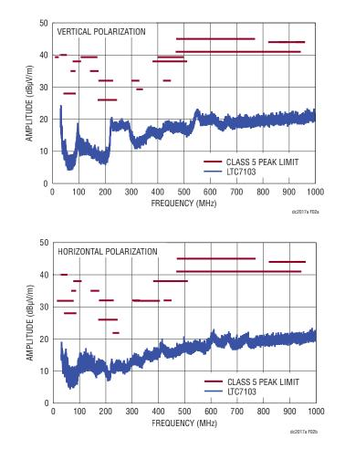
Figure 2. EMI Performance in CISPR 25 Radiated Emission Test (48V<sub>IN</sub> from +VIN\_EMI Turret Pin, 5V<sub>OUT</sub>/2A, f<sub>SW</sub> = 400kHz)
