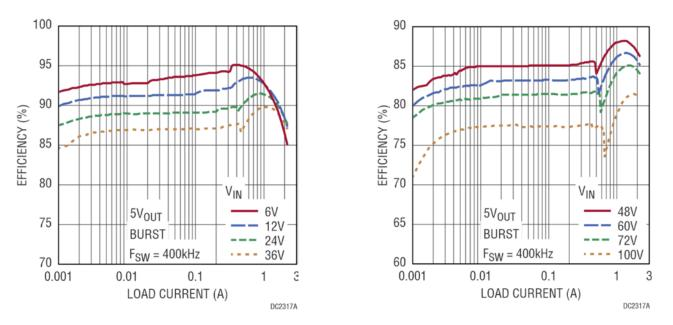
Figure 3. Efficiency at Various Input Voltages (Conditions: Burst Mode Operation)
