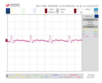
Figure 5. Output Ripple at 100V  $_{\rm IN},\,5V_{\rm OUT}$  and 2.3A  $_{\rm OUT}$  (50mV, 500ns/DIV, 20MHz Bandwidth)
