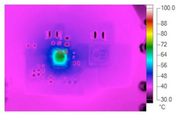
Conditions:  $12V_{IN},\,5V_{OUT}$  at  $2.3A_{OUT}$
