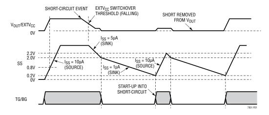
Figure 1. Regulator Shutdown Operation
