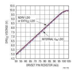
Figure 9. Relationship Between DRV<sub>CC</sub> Voltage and Resistor Value at DRVSET Pin
