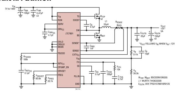
Figure 13. High Efficiency 140V to 12V Step-Down Regulator
