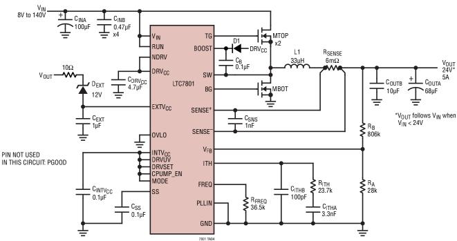
MTOP, MBOT: BSC520N15NS3G D<sub>EXT</sub>: DIODES INC. SMAZ12-13-F L1: WURTH 7443633300 C<sub>OUTA</sub>: SUNCON 35CE68LX D1: NEXPERIA PNE20010ER
