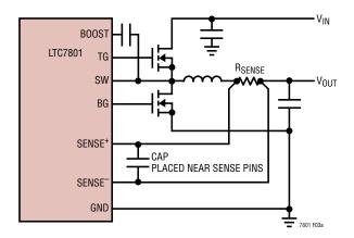
(3a) Using a Resistor to Sense Current
