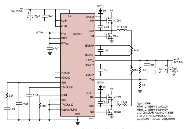
Figure 12. High Efficiency 360W 2-Phase Single Output 12V Step-Down Regulator
