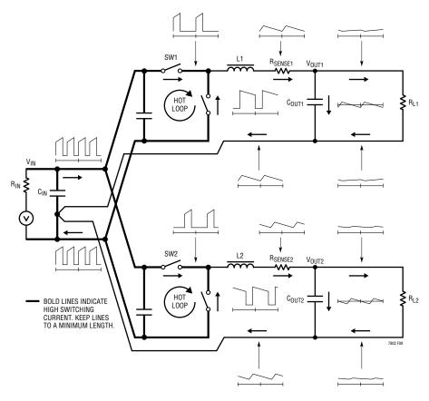
Figure 8. Branch Current Waveforms for Bucks
