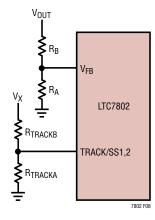
Figure 7. Using the TRACK/SS Pin for Tracking
