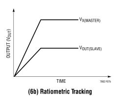
Figure 6. Two Different Modes of Output Voltage Tracking
