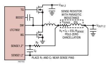
(2a) Using a Resistor to Sense Current
