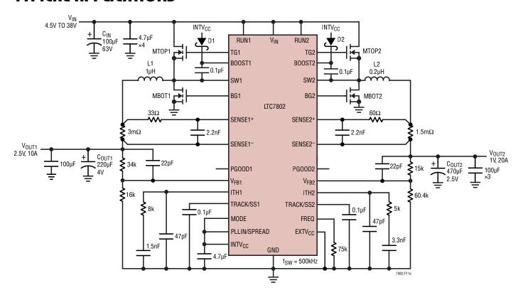
L1: WURTH 744311100 L2: WURTH 744308020 C<sub>OUT1</sub>: KEMET T520V227M004ATE007 C<sub>OUT2</sub>: KEMET T520V477M2R5ATE006 C<sub>IN</sub>: SUNCON 63HVPF100M MTOP1: VISHAY SIR426DP MTOP2: VISHAY SIJA72ADP MBOT1,2: VISHAY SIR640ADP D1,2: CENTRAL SEMI CMDSH-4E
