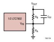
Figure 4. Setting Output Voltage
