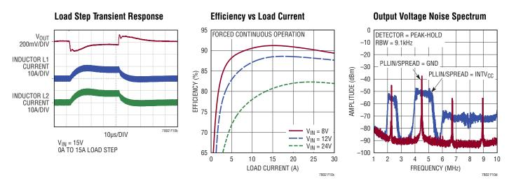
Figure 10. 2.25MHz 2-Phase Single Output 3.3V, 24A Step-Down Regulator
