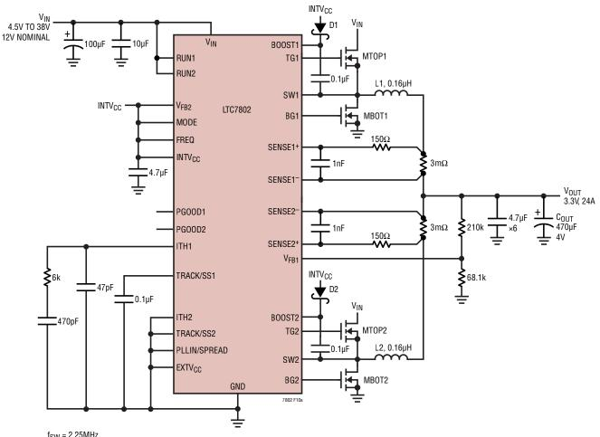
f<sub>SW</sub> = 2.25MHz MTOP1,2: INFINEON BSC059N04LS6 MBOT1,2: INFINEON BSC022N04LS6 L1,2: COILCRAFT XAL5030-161ME D1,2: INFINEON BAS140WE6327HTSA1 C<sub>OUT</sub>: KEMET T520D477M004ATE012
