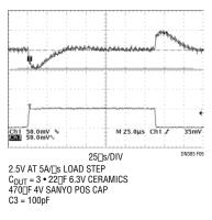
Figure 5. Load Transient Response for the Application in Figure 2
