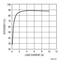
Figure 3. Efficiency of the Application in Figure 2
