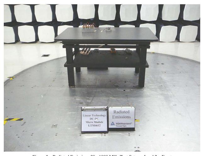
Figure 5 – Radiated Emissions 30 - 1000 MHz Test Setup – Load 2 – Front
