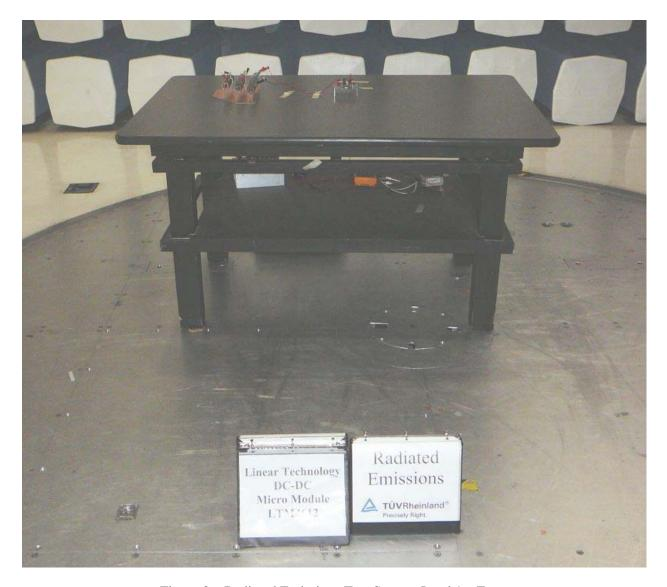
Figure 3 – Radiated Emissions Test Setup – Load 1 – Front
