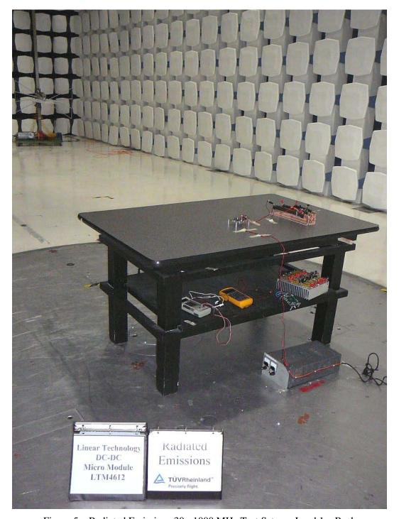
Figure 5 – Radiated Emissions 30 - 1000 MHz Test Setup – Load 1 – Back
