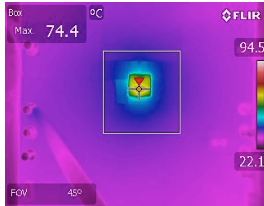
Figure 6. V_{IN} = 5V , V_{OUT} = 3.3V / 5A, T_A = 25C Thermals
