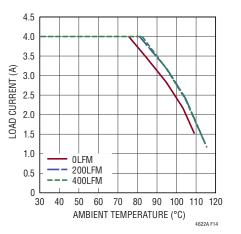
Figure 14. 12V Input to to 1.5V Output Derating Curve, No Heat Sink
