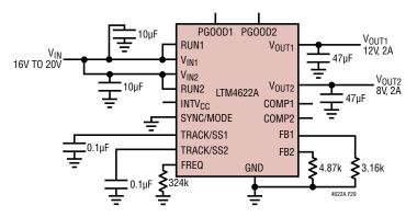
Figure 29. 16V  $_{\rm IN}$  to 20V  $_{\rm IN},$  12V and 8V Output at 2A with 2MHz Switching Frequency
