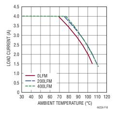
Figure 18. 16V Input to 3.3V Output Derating Curve, No Heat Sink
