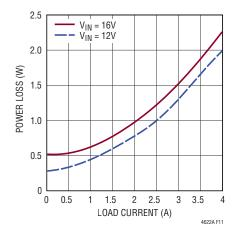
Figure 11. 8V Output Power Loss
