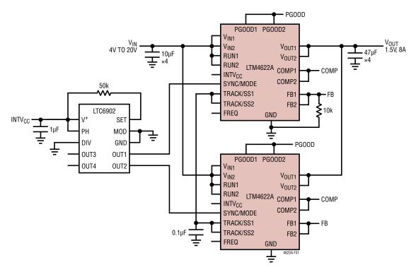
Figure 31. 4 Phase, 1.5V Output at 8A Design with LTC6902
