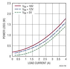
Figure 8. 1.5V Output Power Loss
