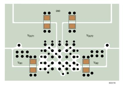
Figure 26. Recommended PCB Layout
