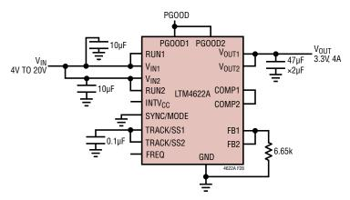
Figure 28.  $4V_{IN}$  to  $20V_{IN}$ , 3.3V Two Phase in Parallel 4A Design
