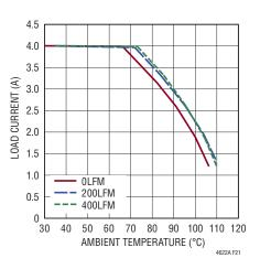
Figure 21. 12V Input to 8V Output Derating Curve, No Heat Sink
