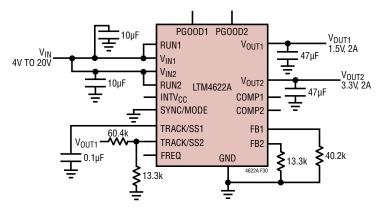
Figure 30.  $4V_{IN}$  to  $20V_{IN}$ , 1.5V and 3.3V Output at 2A Design with Output Coincident Tracking
