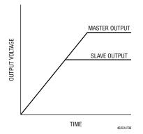
Figure 6. Output Coincident Tracking Waveform
