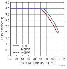
Figure 13. 5V Input to 1.5V Output Derating Curve, No Heat Sink
