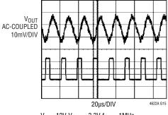
$V_{IN}$  = 12V,  $V_{OUT}$  = 3.3V,  $f_{SW}$  = 1MHz output capacitor = 10  $\mu$ F + 47  $\mu$ F POSCAP
