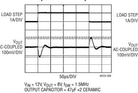
OUTPUT CAPACITOR =  $47\mu$ F ×2 CERAI 10pF FEED-FORWARD CAPACITOR LOAD-STEP = 1A TO 2A (10A/us)
