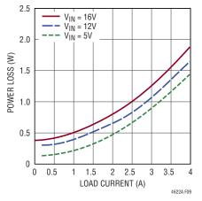
Figure 9. 3.3V Output Power Loss
