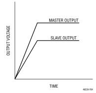
Figure 4. Output Ratiometric Tracking Waveform
