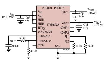
Figure 5. Example Schematic of Ratiometric Output Voltage Tracking
