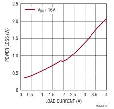
Figure 12. 12V Output Power Loss
