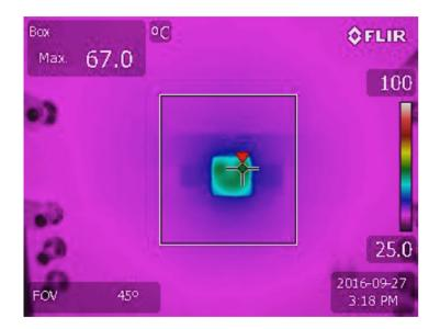
Figure 24. Thermal Image, 12V Input, 3.3V and 5V Output, 2A Each, No Airflow and No Heat Sink
