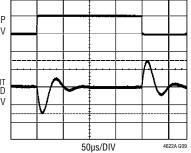
$\begin{array}{l} V_{IN} = 16V, \ V_{OUT} = 12V, \ f_{SW} = 1.5MHz \\ 0UTPUT \ CAPACITOR = 47 \mu F \times 2 \ CERAMIC \\ 10pF \ FEED-FORWARD \ CAPACITOR \\ I \ OAD-STEP = 1A \ TO \ 2A \ (10A/us) \end{array}$
