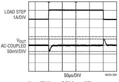
$\label{eq:VIN} \begin{array}{l} V_{IN} = 12V, \ V_{OUT} = 3.3V, \ f_{SW} = 1MHz \\ OUTPUT \ CAPACITOR = 47\mu F \times 1 \ CERAMIC \\ 10pF \ FEED-FORWARD \ CAPACITOR \\ LOAD-STEP = 1A \ TO \ 2A \ (10A/\mu s) \end{array}$
