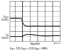
$V_{IN}$  = 12V,  $V_{OUT}$  = 3.3V,  $f_{SW}$  = 1MHz output capacitor = 10  $\mu F$  ceramic + 47  $\mu F$  Poscap
