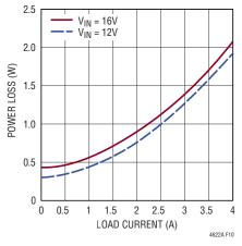
Figure 10. 5V Output Power Loss
