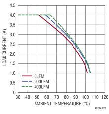
Figure 23. 16V Input to 12V Output Derating Curve, No Heat Sink
