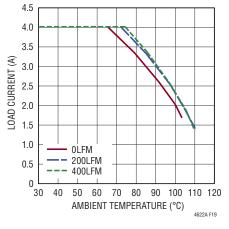
Figure 19. 12V Input to 5V Output Derating Curve, No Heat Sink
