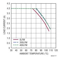
Figure 17. 12V Input to 3.3V Output Derating Curve, No Heat Sink
