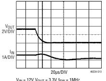
$V_{IN}$  = 12V,  $V_{OUT}$  = 3.3V,  $f_{SW}$  = 1MHz output capacitor = 10  $\mu$ F + 47  $\mu$ F Poscap
