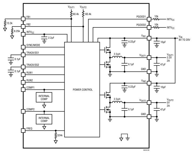
Figure 1. Simplified LTM4622A Block Diagram
