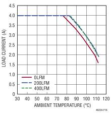
Figure 16. 5V Input to 3.3V Output Derating Curve, No Heat Sink
