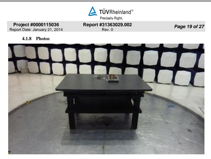
Figure 4 - Radiated Emissions Test Setup 30 - 1000 MHz - Front
