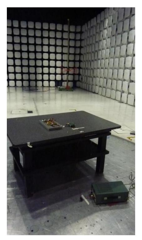
Figure 5 - Radiated Emissions Test Setup 30 - 1000 MHz - Back
