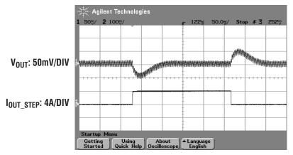
3a.  $V_{\text{IN}}$  = 12V,  $V_{0}$  = 3.3V, 0A to 4A Load Step
