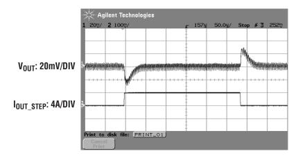
3b.  $V_{\text{IN}}$  = 12V,  $V_0$  = 1.0V, 0A to 4A Load Step
