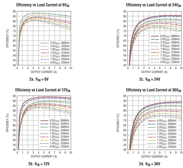
Figure 2. Measured DC1543A Efficiency at Different  $V_{IN}$ ,  $V_{OUT}$  and  $f_{SW}$  (CCM Mode Enabled) Please refer to Table 1 in LTM4641 data sheet for the switching frequency at each output voltage.
