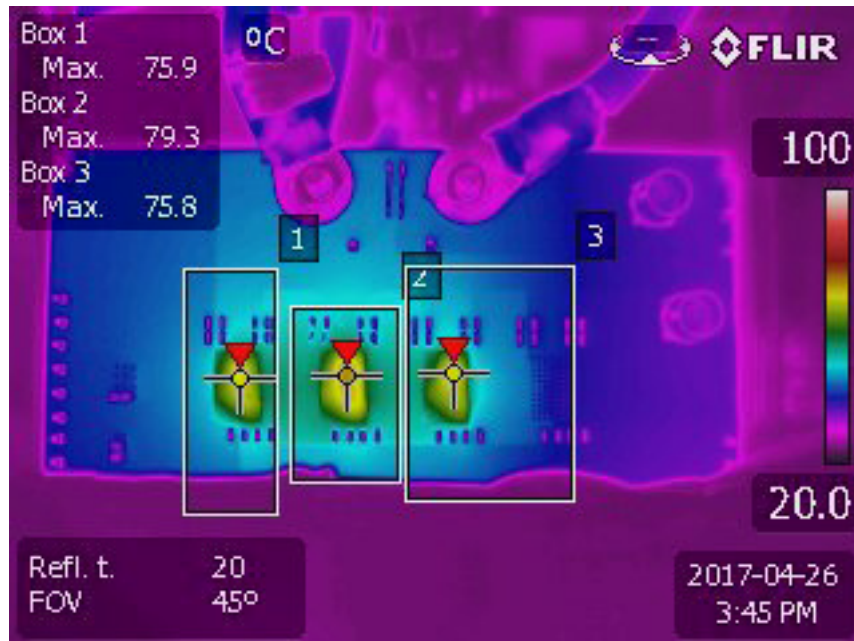
Figure 4. Thermal Capture at 12V IN , 1.0V OUT , 75A (T A = 25°C, 200LFM Airflow and No Heat Sink)
