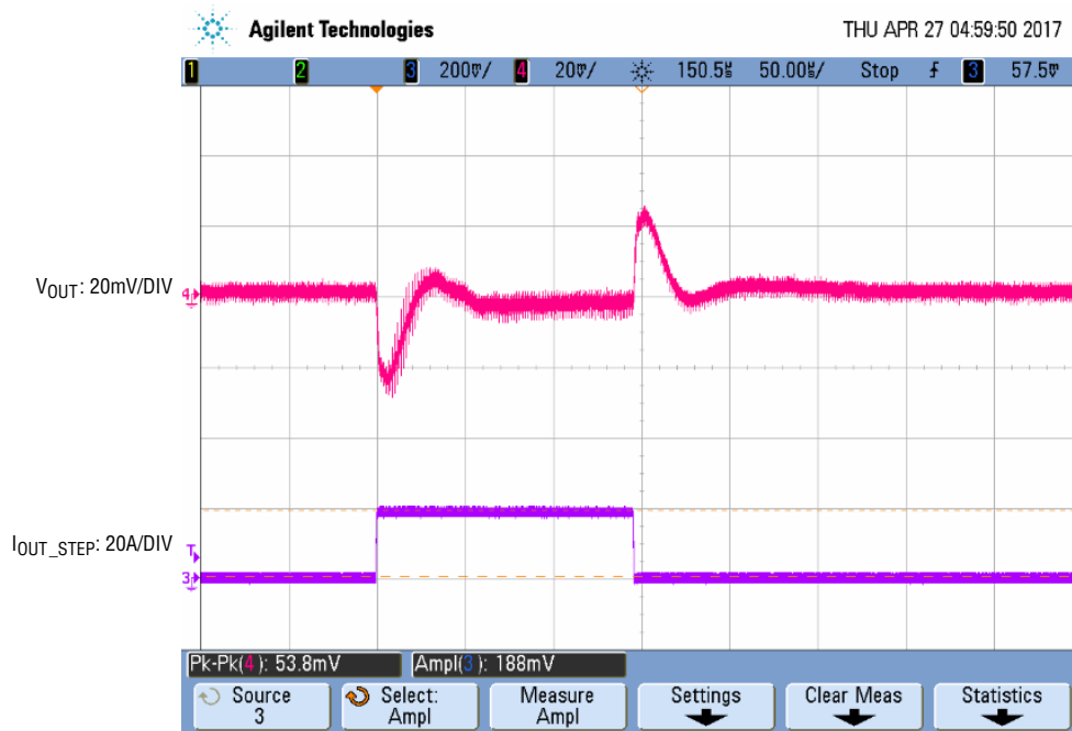
Figure 3. Measured Load Transient V IN = 12V, V OUT = 1.0V, I STEP = 0A to 18.75A
