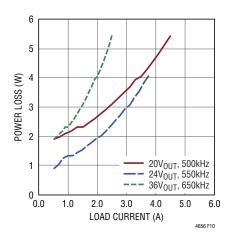
Figure 10. Power Loss vs Load Current 12V<sub>IN</sub> Based on LTM4656
