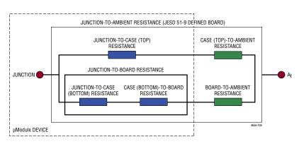
Figure 8. Graphical Representation of JESD51-12 Thermal Coefficients
