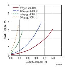
Figure 9. Power Loss vs Load Current 5V<sub>IN</sub> Based on LTM4656
