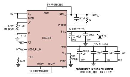
Figure 19. 5V Input to 12V  $_{\hbox{\scriptsize OUT}}$  at 3.25A Design
