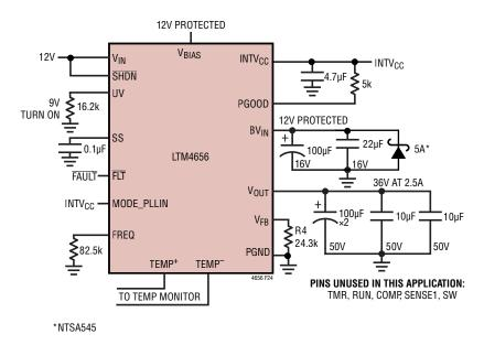
Figure 24. 12V Input to 36V<sub>OUT</sub> at 2.5A Design
