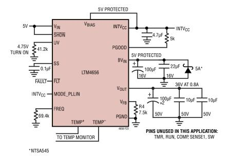
Figure 23. 5V Input to 36V<sub>OUT</sub> at 0.8A Design
