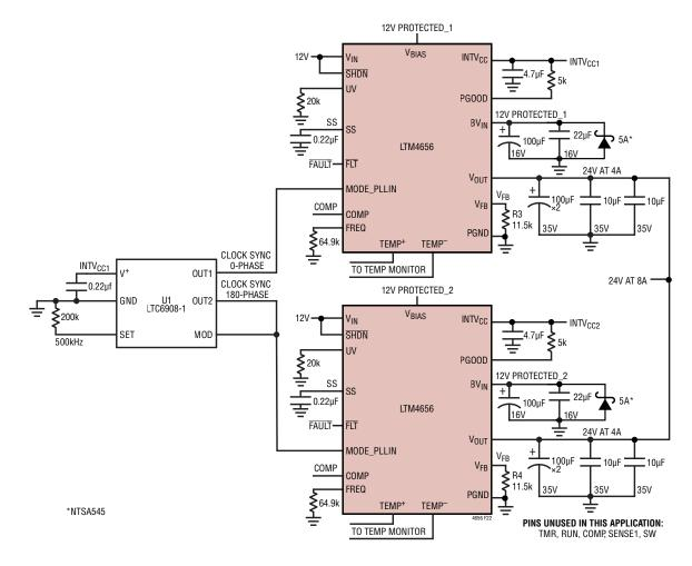
Figure 22. 2-Phase 12V Input to 24V<sub>OUT</sub> at 8A Design
