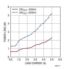
Figure 11. Power Loss vs Load Current 24V<sub>IN</sub> Based on LTM4656
