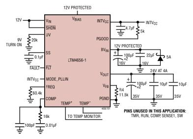
Figure 21. 12V Input to 24V<sub>OUT</sub> at 4A Design
