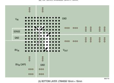
Figure 18. Recommended PCB Layout
