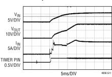
24V to 36V Boost HOT Plugged Start-Up Into 5A Load
