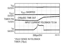
Figure 4. 10V Input to 36V Output Short Input Current Trip Waveform
