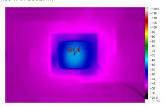
Figure 7. 12V<sub>IN</sub> to 24V<sub>OUT</sub> at 4A (96W), 200LFM Air Flow Thermal Plot
