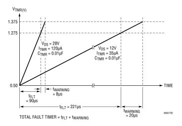
Figure 2. Overcurrent Fault Time with 0.01µF
