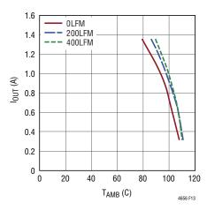
Figure 13. LTM4656  $5V_{IN}$  24 $V_{OUT}$  500kHz no HS
