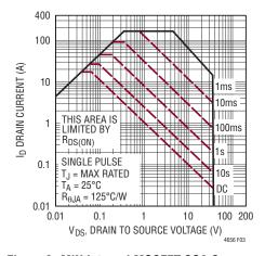
Figure 3. MIN Internal MOSFET SOA Curves
