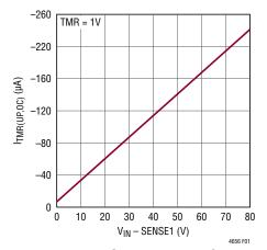
Figure 1. Overcurrent TMR Current vs V<sub>IN</sub> – SENSE1 Voltage
