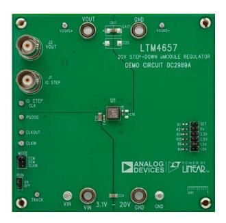
Demonstration circuit 2989A is an easy way to evaluate the performance of the LTM4657. Please refer to Figure 1 for test setup connections and follow the procedure below.
