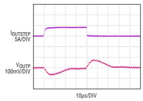
Figure 3. Load Transient (4A to 8A) Response Waveform at  $12V_{\text{IN}}$  and 1.5Vout, 10 $\mu\text{s}/\text{div}$
