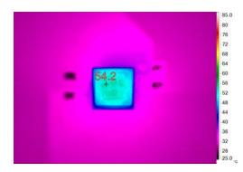
Figure 4. Measured Thermal Capture at  $12V_{IN}$  and  $1.5V_{OUT},\,8A_{OUT}$  at 25°C Ambient with No Airflow
