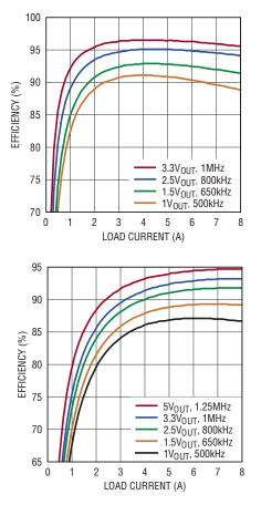
Figure 2. Measured Supply Efficiency at  $5V_{\text{IN}}$  and  $12V_{\text{IN}}$
