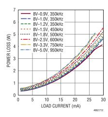
Figure 12. 8V<sub>IN</sub> Power Loss Curve
