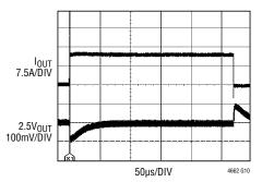
$C_{OUT}$  = 100 $\mu$ F ×2, CERAMIC  $C_{COMP}$  = 100 $\rho$ F,  $C_{FF}$  = 47 $\rho$ F f = 500kHz
