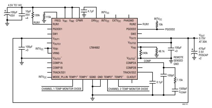
Figure 21. 12V Input to 0.75V at 30A Two Phase
