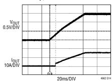
$\begin{array}{l} 12V_{IN}, 1.5V_{OUT} \text{ AT } 15\text{A LOAD} \\ C_{OUT} = 470\mu\text{F} \times 1, 2.5\text{V}, \text{SANYO POSCAP}, \\ 100\mu\text{F} \times 4, 6.3\text{V}, \text{CERAMIC} \\ \text{SOFT-START CAPACITOR} = 0.1\mu\text{F} \\ \text{USE RUN PIN TO CONTROL START-UP} \end{array}$
