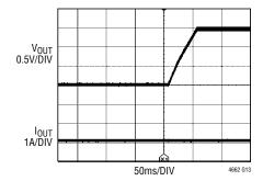
$12V_{IN},\,1.5V_{OUT}$  AT NO LOAD  $C_{OUT}=470\mu F\times 1,\,2.5V,\,SANYO$  POSCAP,  $100\mu F\times 4,\,6.3V,\,CERAMIC$  SOFT-START CAPACITOR =  $0.1\mu F$  USE RUN PIN TO CONTROL START-UP
