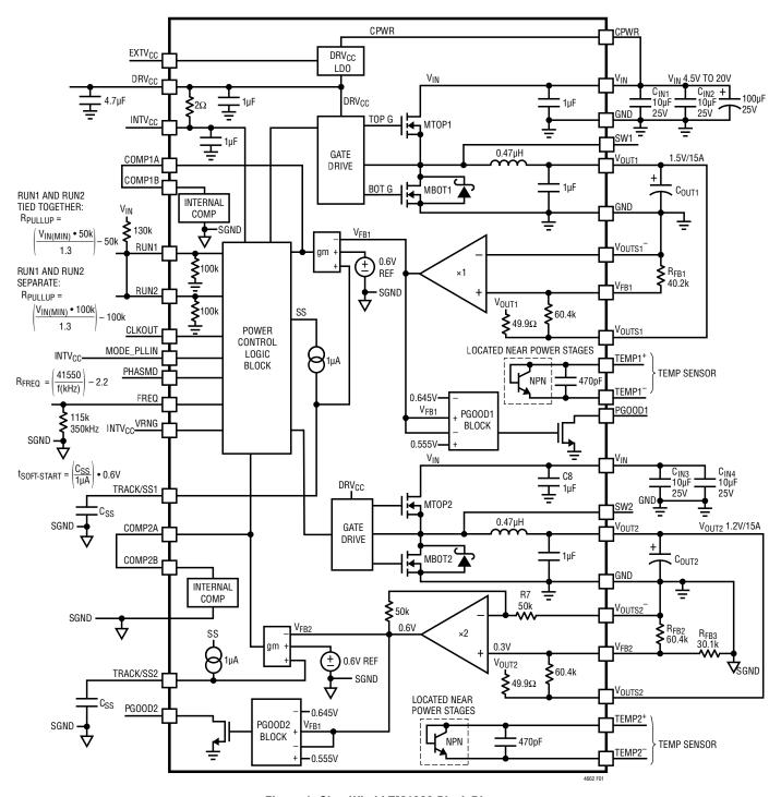
Figure 1. Simplified LTM4662 Block Diagram
