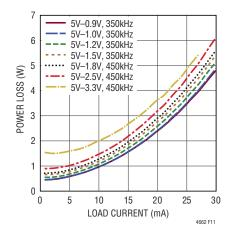
Figure 11. 5V<sub>IN</sub> Power Loss Curve
