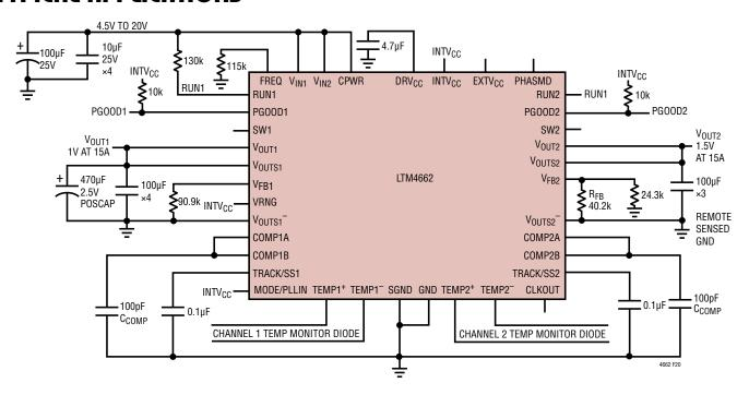
Figure 20. 4.5V to 20V Input to 1.0V and 1.5V at 15A Each
