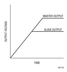
Figure 6. Output Coincident Tracking Waveform
