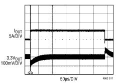
$C_{OUT}$  = 100 $\mu$ F ×1, CERAMIC  $C_{COMP}$  = 100pF,  $C_{FF}$  = 47pF f = 750kHz
