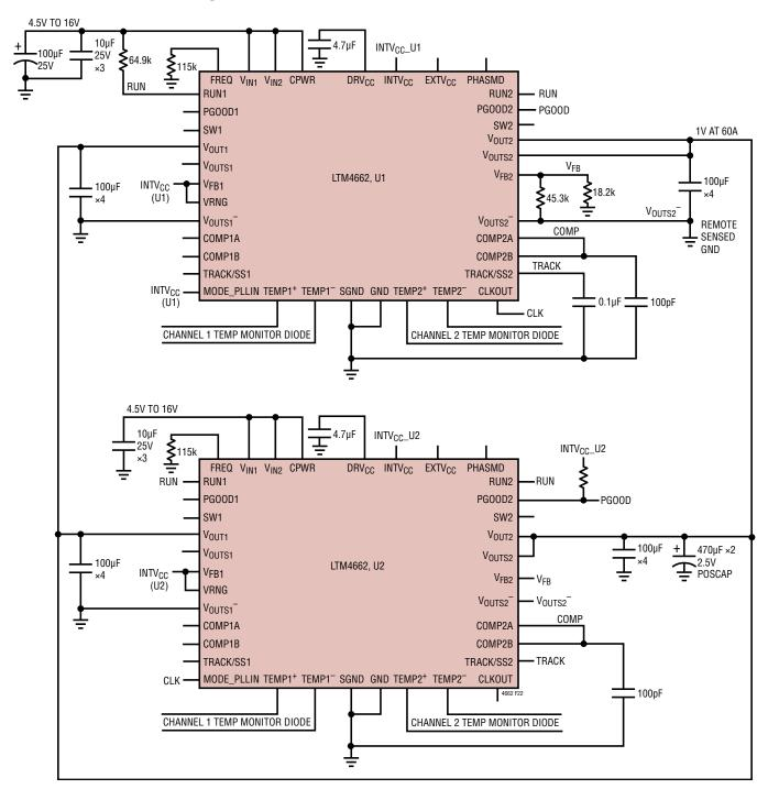
Figure 22. Four Phase Design 1V at 60A
