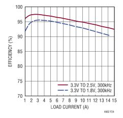
Figure 24. Efficiency, 3.3V<sub>IN</sub>
