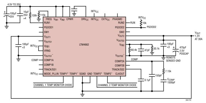
Figure 2. 2-Phase Parallel Configurations
