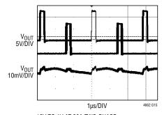
12V TO 1V AT 30A TWO-PHASE 12V TO 1V AT 350kHz RIPPLE AT 30A LOAD  $C_{OUT}$  = 330 $\mu$ F, 9m $\Omega$ , 100 $\mu$ F ×4, CERAMIC
