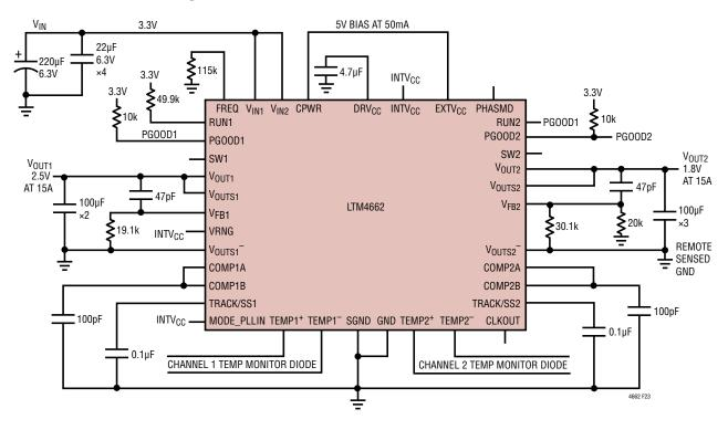
Figure 23. 3.3V to 1.8V, and 2.5V at 15A each with PGOOD Power Up Sequencing
