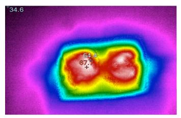
Figure 10. LTM4662 12V to 5V at 22A with 400LFM, 30°C Ambient, 110W
