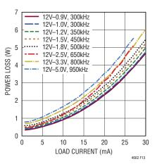
Figure 13. 12V<sub>IN</sub> Power Loss Curve
