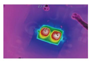
Figure 9. LTM4662 12V to 1V at 30A with 400LFM, 30°C Ambient, 30W
