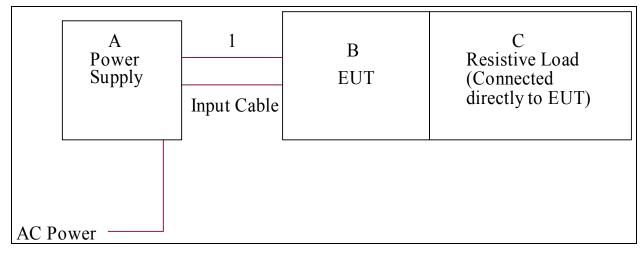
Figure 1. Block Diagram of Test Configuration
