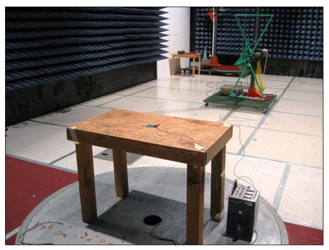
Photograph 1. Radiated Emission: Limits of Electromagnetic Radiation Disturbance, Test Setup
