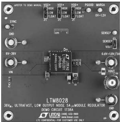
Figure 2. The LTM8028 Makes It Possible to Build a Minimal Component-Count Regulator That Meets Stringent Noise, Efficiency and Transient Response Requirements
