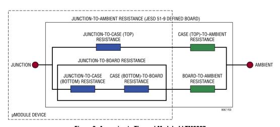
Figure 3. Approximate Thermal Model of LTM8067
