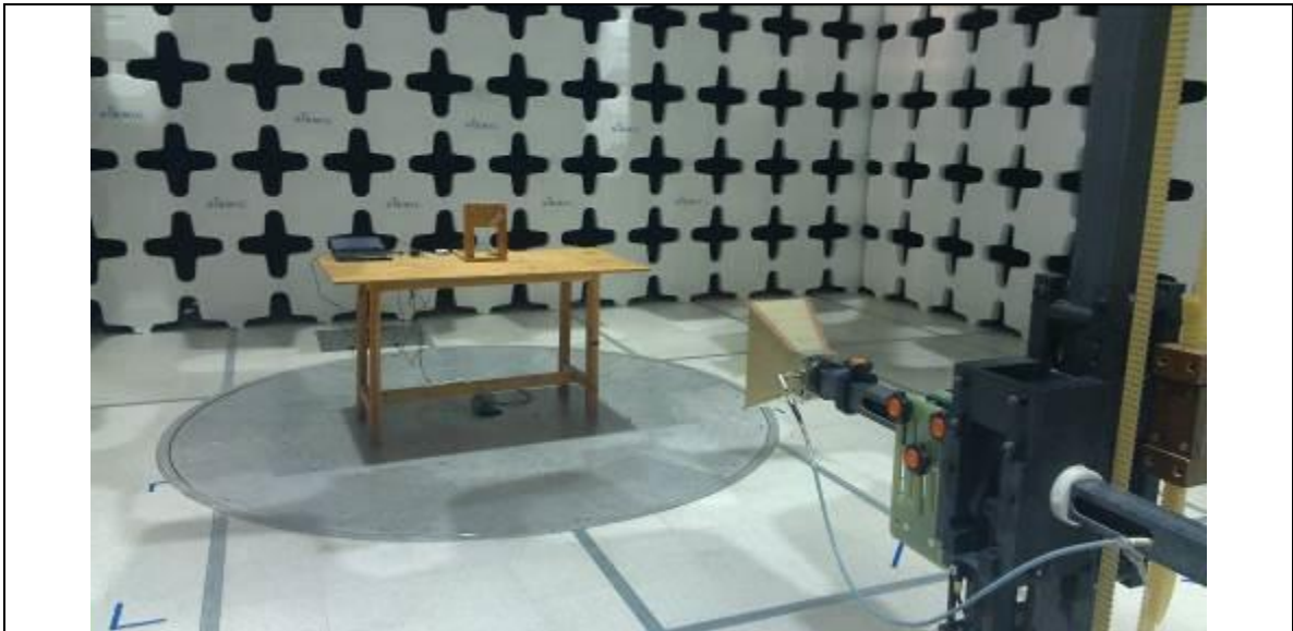
Radiated Emission Test Setup (above 1GHz) with Chip antenna- Front View
