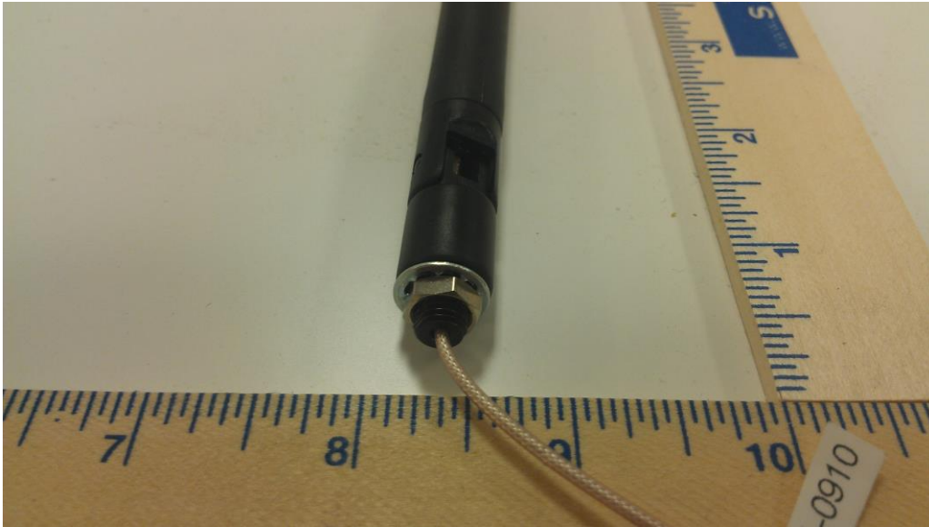
5dBi dipole antenna (Nearson_S151FL-L-RMM-2450S) – Port view
