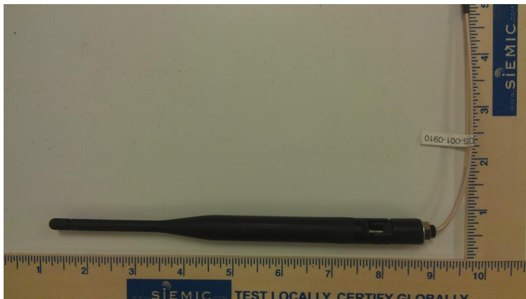
5dBi dipole antenna (Nearson_S151FL-L-RMM-2450S) – Top view
