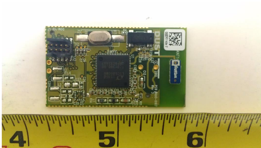
Radio module ((LTP5901) without shielding
