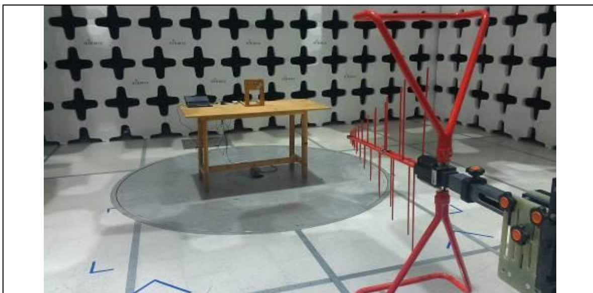
Radiated Emission Test Setup (below 1GHz) with Chip antenna - Front View
