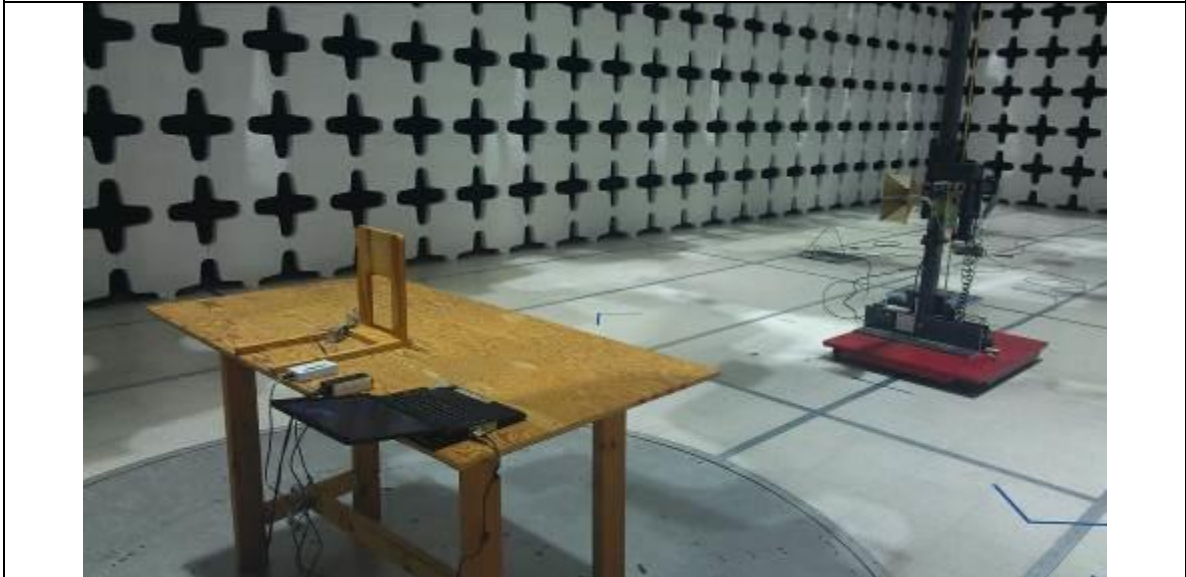
Radiated Emission Test Setup (above 1GHz) with Chip antenna – Rear View
