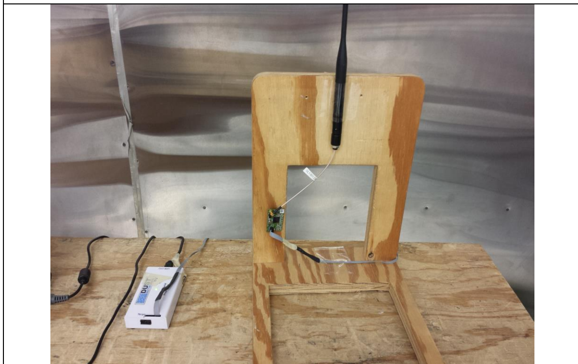
Close view of test configuration - with 5 dBi dipole antenna -2
