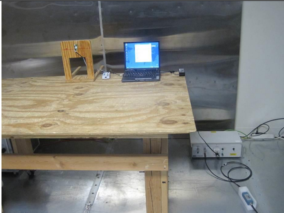
Conducted Emission Setup Front View (AC Line)- Front View
