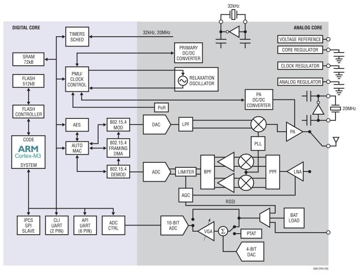
Figure 5. Eterna Block Diagram
