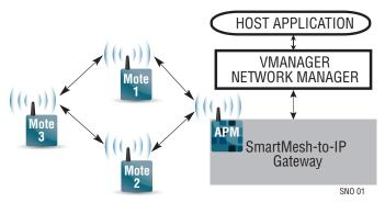
An ongoing discovery process ensures that the network continually discovers new paths as the RF conditions change. In addition, each mote in the network tracks performance statistics (e.g. quality of used paths, and lists of potential paths) and periodically sends that information to the network manager in packets called health reports. The network manager uses health reports to continually
