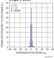
TIMEn Synchronization Error 1 Packet/s Publishing Rate, 5 Hops, 2°C/Min.
