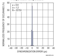
TIMEN Synchronization Error 1 Packet/s Publishing Rate, 3 Hops, Room Temperature
