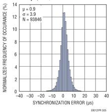
TIMEn Synchronization Error 0 Packet/s Publishing Rate, 3 Hops, 8°C/Min.
