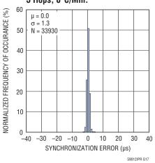
TIMEn Synchronization Error 1 Packet/s Publishing Rate, 5 Hons 8°C/Min
