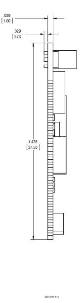
Figure 14. LTP5902 Mechanical Drawing
