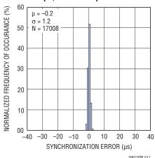
TIMEN Synchronization Error 1 Packet/s Publishing Rate, 5 Hops, Room Temperature
