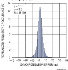
TIMEn Synchronization Error O Packet/s Publishing Rate, 5 Hops, Room Temperature
