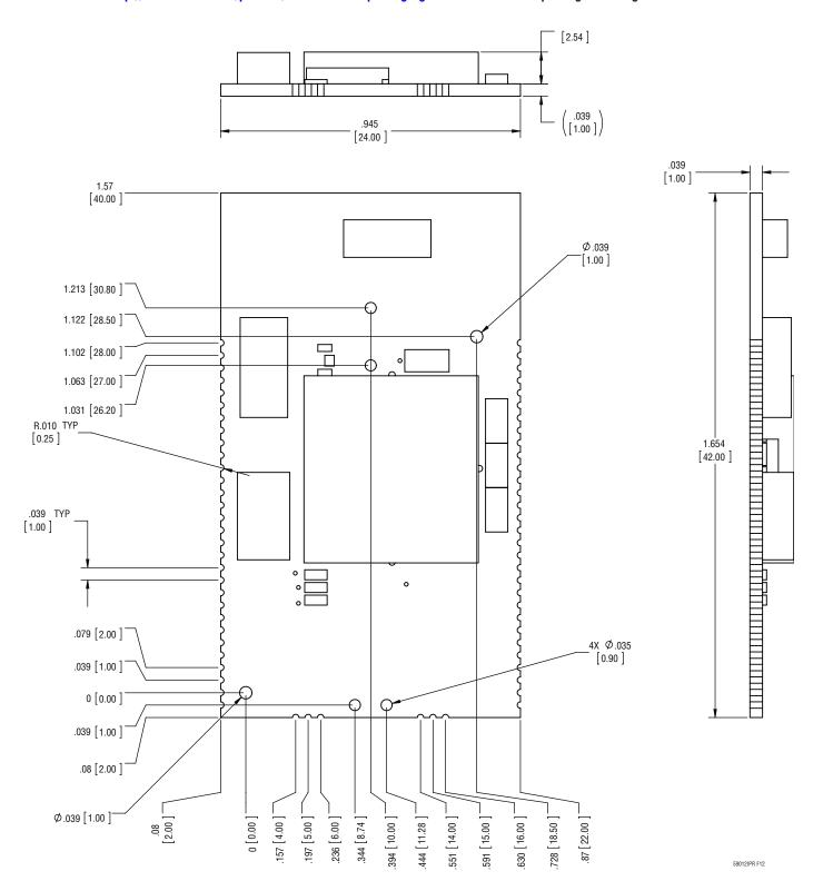
Figure 13. LTP5901 Mechanical Drawing
