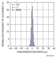
TIMEn Synchronization Error O Packet/s Publishing Rate, 3 Hops, 2°C/Min.
