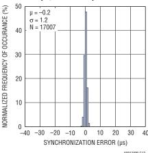
TIMEn Synchronization Error 1 Packet/s Publishing Rate, 1 Hop, 2°C/Min.
