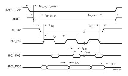
Figure 2. Flash Programming Interface Timing
