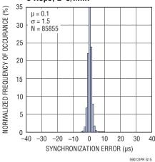
TIMEn Synchronization Error 1 Packet/s Publishing Rate, 1 Hop, 8°C/Min.
