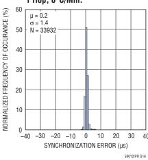
TIMEn Synchronization Error 1 Packet/s Publishing Rate, 3 Hops, 8°C/Min.
