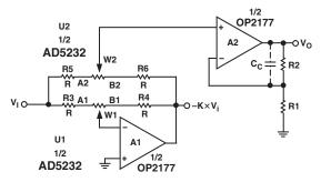
Figure 3. PGA Handles High Input Voltage
