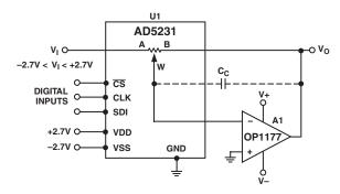
Figure 1. Programmable Amplifier/Attenuator
