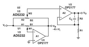
Figure 2. Bipolar Programmable-Gain Amplifier with Linear Step Adjustment
