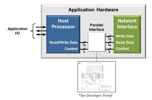
Figure 8 – Parallel Host Interface Connection
