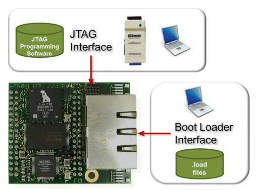
Figure 9 – Programming Connections and Devices
