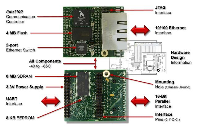
Figure 1 – Overview of Module Components and Interfaces
