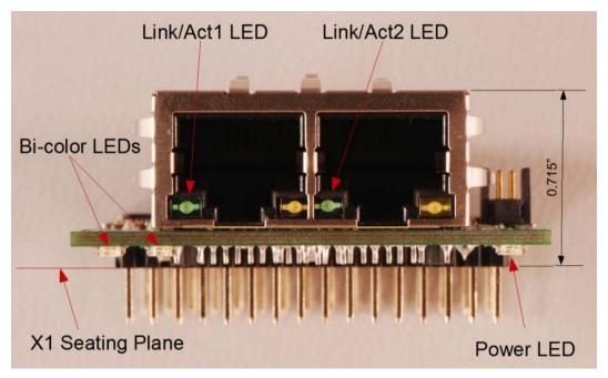
Figure 3 - Dimensions of the Network Interface Module (Cross-section)
